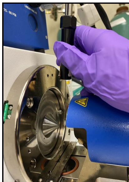
Figure 5.2 DART-HRMS analysis of SPME fiber.
