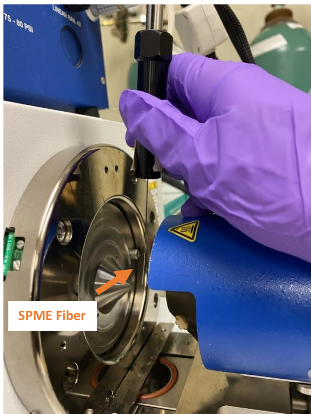
Figure 1.8 SPME fiber suspended between the DART ion source and the MS inlet (while being held using a SPME fiber holder). Analytes adsorbed to the fiber are desorbed in the heated DART gas stream and ionized before entering the MS inlet.
