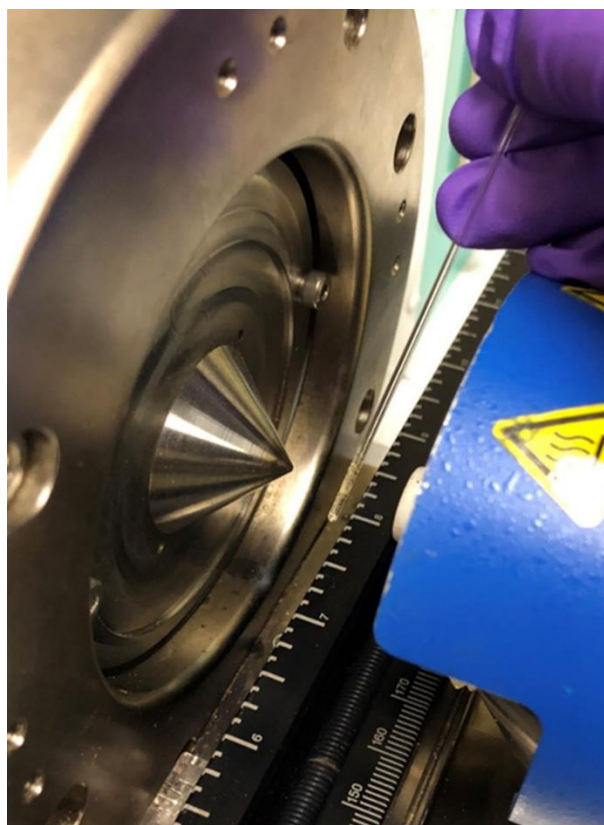
Figure 1.7 Capillary tube suspended between the DART ion source and the MS inlet after being exposed to a powdered sample.
