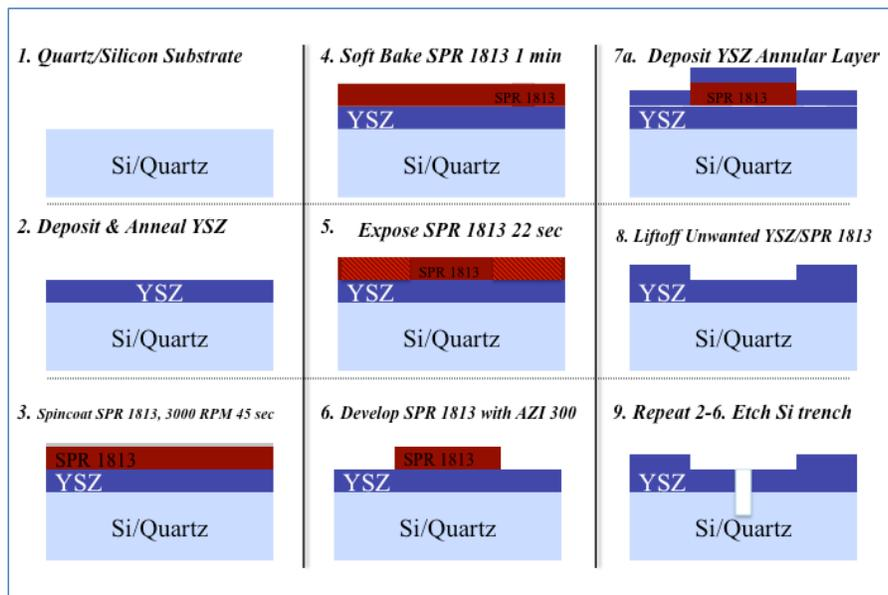
Figure 6 Chamber Component Fabrication Process Layout
