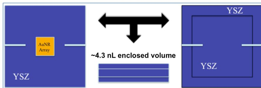
Figure 1 Both Components of the nanoliter reaction chamber bonded together
