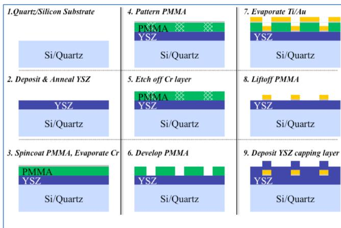
Figure 4 Nanorod Patterning Process Steps
